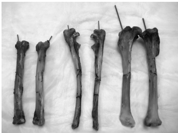
FIGURE 1. Examples of paired canine radii, ulnas, and tibias used in the study with implanted flexible IM nails.
